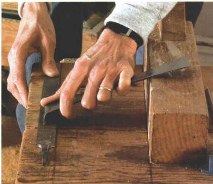
A 4x4 guides flat scraper. Running the tail end of a combination scraper/pry bar along a block of wood allows the author to maintain a consistent sharpening angle. Pencil lines on the bench top ensure correct placement of the block and the file.
