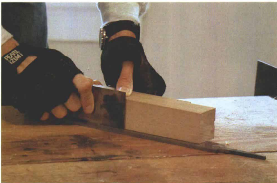
Square stock guides cabinet scraper. On the job site, the author quickly restores a usable edge on a scraper by running it across the top of the file with a square wooden block as a fence.
