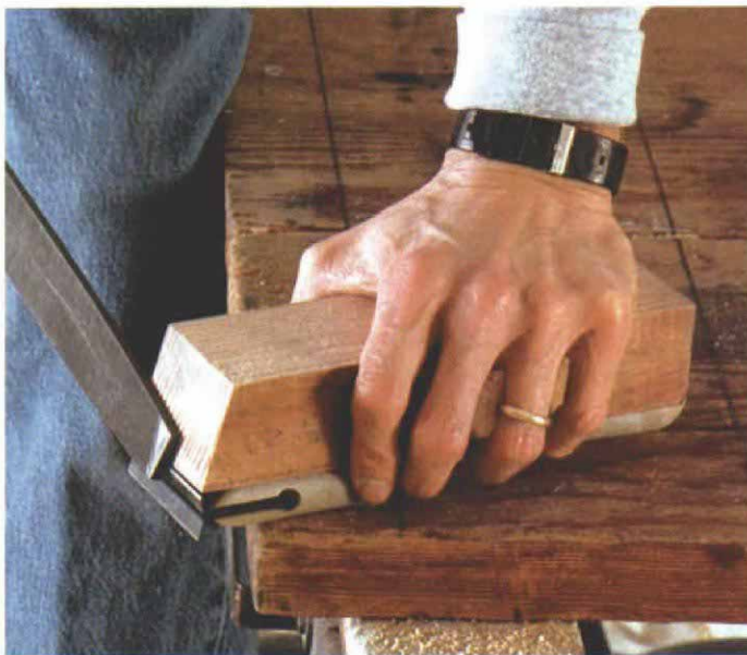
Angled block guides the file. A chunk of scrap maple, cut to the same width as the paint scraper and mitered to match the cutting angle of the blade, keeps the file aligned precisely with the blade.
