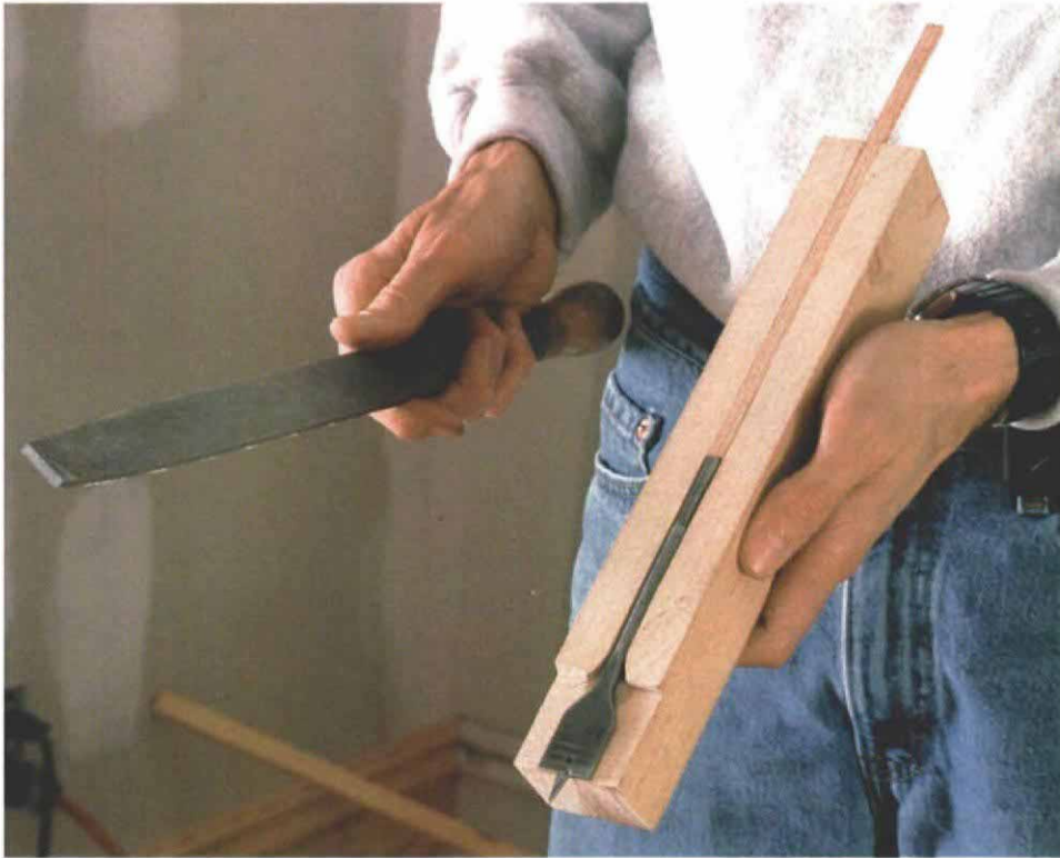
Easier than running to the hardware store every time you hit a nail. This jig (top photo) that clamps to any flat work surface ensures that a sharp, perfectly aligned spade bit is never more than a few file strokes away (photo right).
